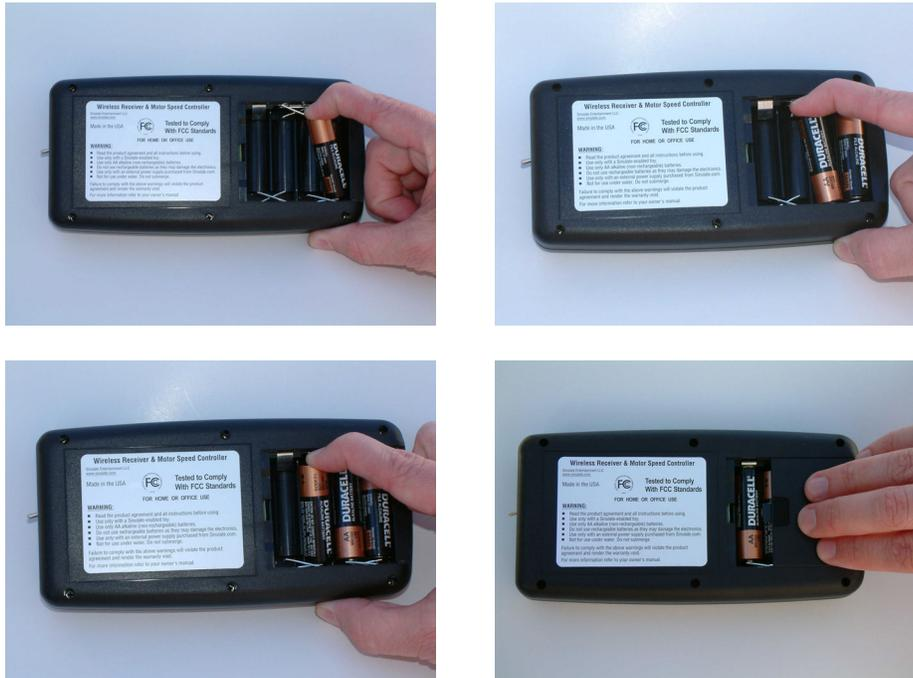
Figure 14 – Battery Installation
