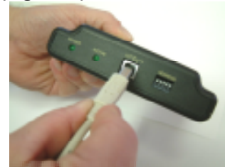
Figure 5 - Connecting the USB Cable
